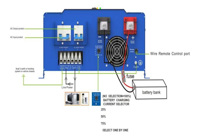
Battery charging current:battery charging current selector on100%(100% is the maximum Battery current) as below
