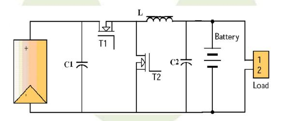
MPPT Module Use DC / DC converter (BUCK Topology structure using synchronous rectification). The maximum power point is found by the maximum power tracking algorithm and the maximum power output of the solar cell is obtained.
